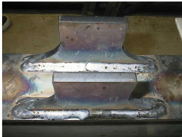
Figure 7.2. Two attachments welded on the beam used in experiment. Note how the weld is uneven and the dark dots on the weld.
